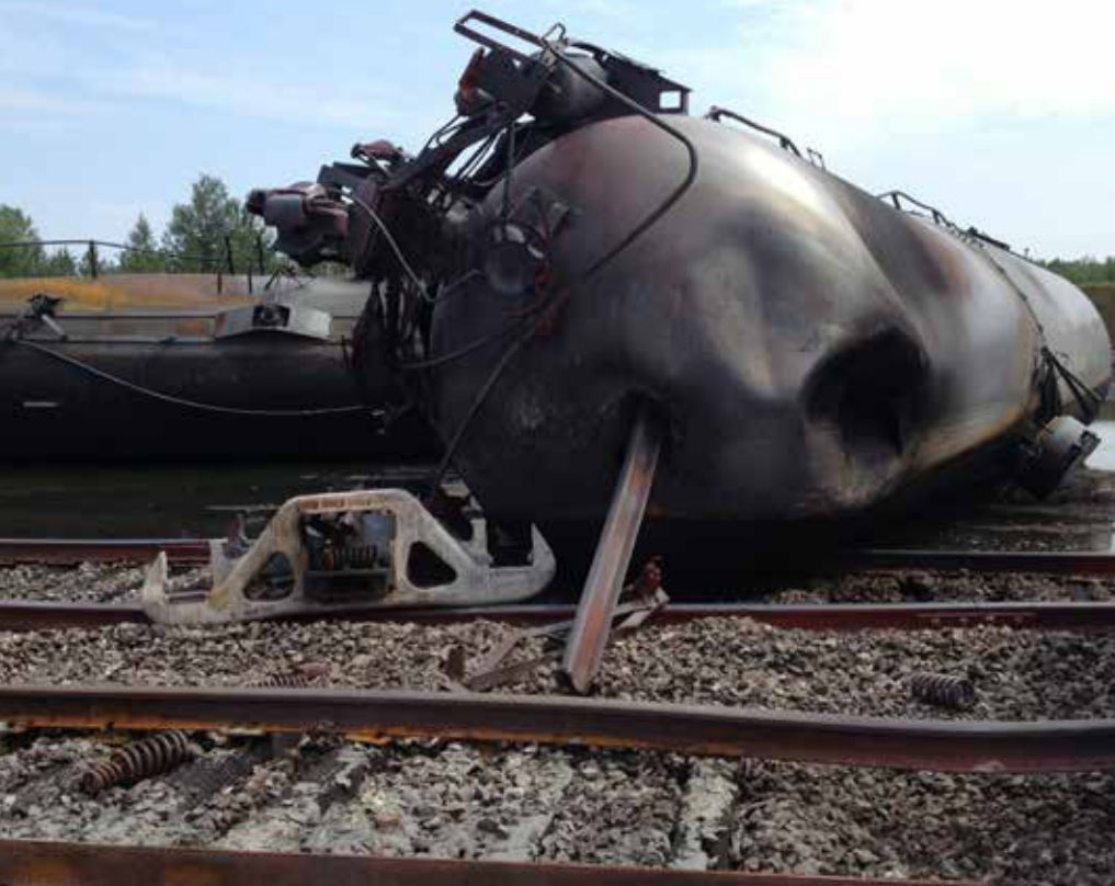
A tank car involved in the Lac-Mégantic wreck displays fire and crash damage, including a rail through the tank's shell. Transportation Safety Board of Canada
